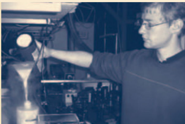
Erik Herz pouring liquid nitrogen to cool the cameras used for single quantum dot spectroscopy in his lab at the University of Dortmund.
